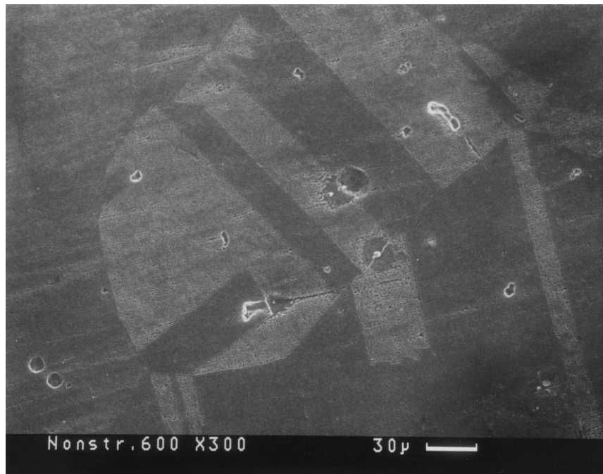
Fig. 3. Autoradiographic microstructure of nonstrained 600 super alloy. Hydrogen is trapped on the interface of inclusion and matrix (A); interface of carbides and matrix (B) and grain boundaries (C). \times 300 .
